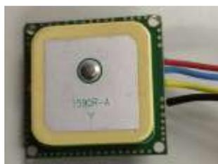
Fig.4 32 Channel LS20031 GPS 5Hz Receiver
